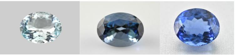
**5.** Examples of classic aquamarine colour (left), saturated blue aquamarine (centre) and maxixe-type blue beryl (right). Saturated colours (centre and right) require detailed absorption spectroscopy for separation of aquamarine and maxixe-type blue beryls.
