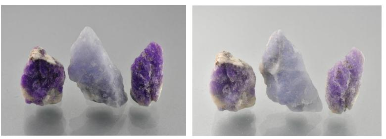
**1.** Rough samples of hackmanite after exposure to UV light (left) and after fading (right. Note the intensification of purple-violet component after exposure to UV light. The sample in centre is least affected by the UV exposure but still display some degree of colour change.
