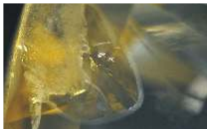
b. Healed Fingerprints / Burst Halo with a glassy reflection &amp; white edges
