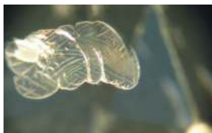
e. Burst halo with a sugary crystal and 'fern-like' pattern formed due to re-crystallisation
