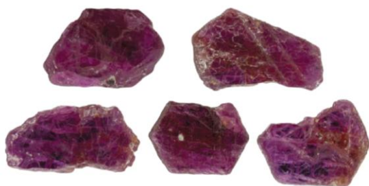
Figure 2: The appearance of these Mozambique rubies are improved by heating and flux-assisted healing of fractures.
