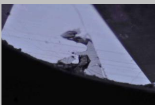
e. Many of these Mozambique rubies have cavities filled with glass, which display duller lustre
