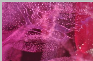
b. Surface breaks typically displays flow and net like patterns
