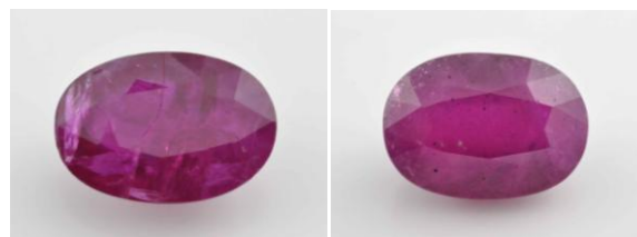
Figure 3: Rubies from Mozambique (heated with flux)-left and Madagascar (lead-glass filled)-right.
