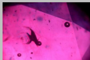
g. Gas bubbles are also a common feature in Lead-glass filled rubies from Madagascar
