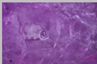
f. Glass-filled cavities often display gas bubbles
